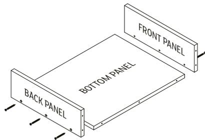
Attach the front and back drawer box panels to the base drawer box panel.
