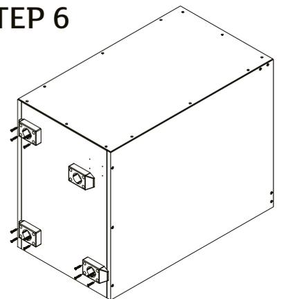
Screw the base plates for the adjustable legs in position.
