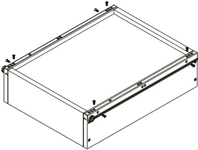
**Note:** The guide wheel end of the drawer runner should be flush with the end of the drawer box.
