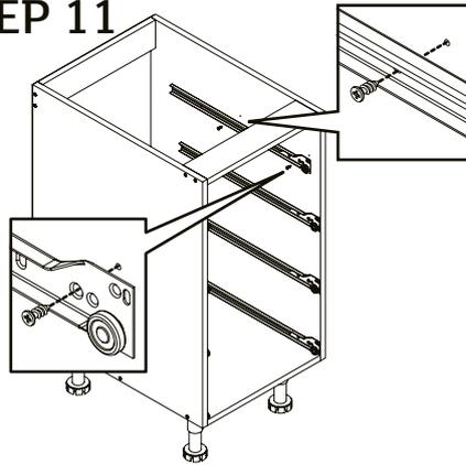
Place drawer runner on the side of the cabinet and align with the predrilled holes. Secure with the 14mm screws provided. Repeat for the remaining drawer runners.
