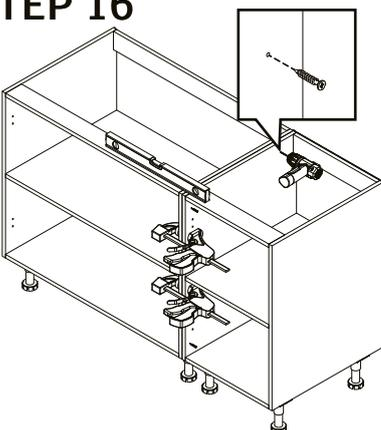
Check cabinets are level then clamp together. Pre-drill using 2mm drill bit and attach cabinets together.
