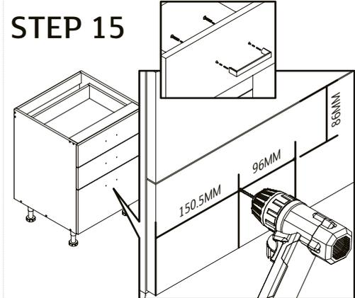
Place masking tape on both sides of the drawer front where holes will be drilled to avoid chipping. Pre-drill using 4.5mm drill bit. Attach handle using the screws provided.
