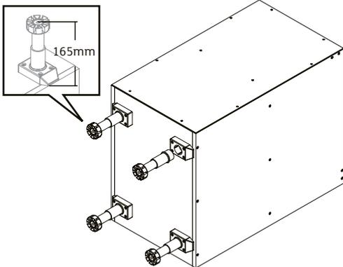
Attach leg to the base plate. Set the height of the adjustable legs to 165mm. Repeat for the remaining legs.
