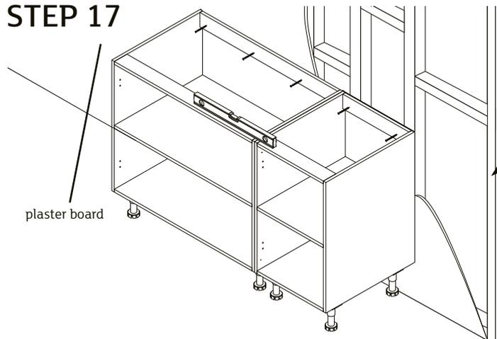
**Caution:** Please ensure all cabinets are screwed into your timber stud wall using a minimum of 60mm timber screws. If attaching to concrete, brick, steel or any other substrates seek advice from your hardware specialist.
