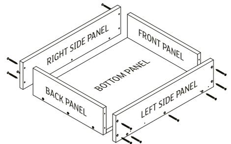
Attach the side panels to the rest of the drawer box. Repeat for the remaining drawers.
