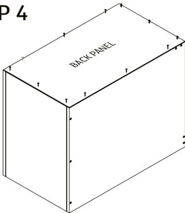
Nail back panel onto the side panels, base panels and fixed shelf. Screw the back panel into the top support rail.
