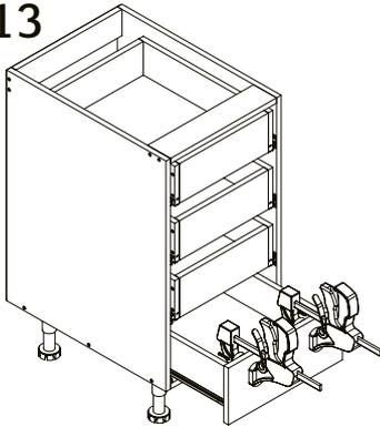
Clamp the drawer front onto the bottom drawer ensuring it is evenly spaced either side and level with the bottom panel of the cabinet. Predrill and attach using the 28mm screws provided.
