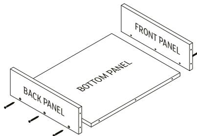
Attach the front and back drawer box panels to the base drawer box panel.
