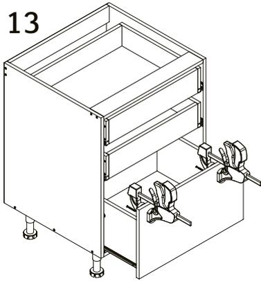
Clamp the drawer front onto the bottom drawer ensuring it is evenly spaced either side and level with the bottom panel of the cabinet. Predrill and attach using the 28mm screws provided.
