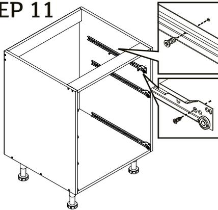
Place drawer runner on the side of the cabinet and align with the predrilled holes. Secure with the 14mm screws provided. Repeat for the remaining drawer runners.
