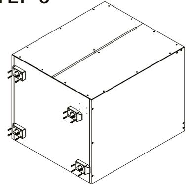
Screw the base plates for the adjustable leg in position.
