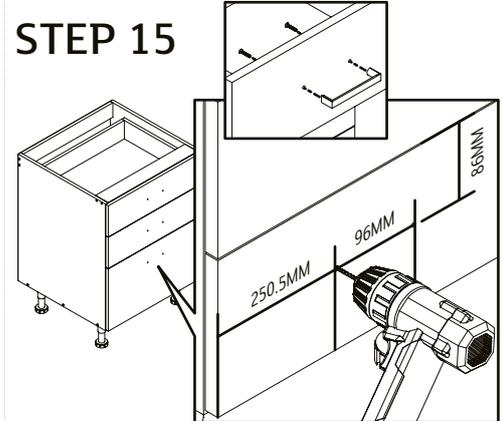
Place masking tape on both sides of the drawer front where holes will be drilled to avoid chipping. Pre-drill using 4.5mm drill bit. Attach handle using the screws provided.
