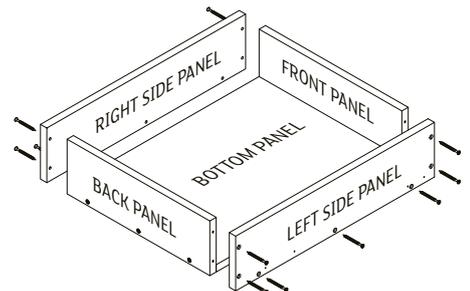
Attach the side panels to the rest of the drawer box. Repeat for the remaining drawers.
