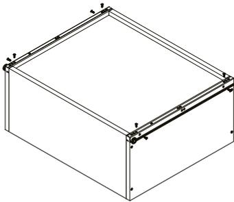
**Note:** The guide wheel end of the drawer runner should be flush with the end of the drawer box.
