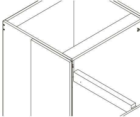
Attach the oven panels to the cabinet using the 90° brackets. The larger panel goes down the bottom whilst the smaller panel goes at the top.
