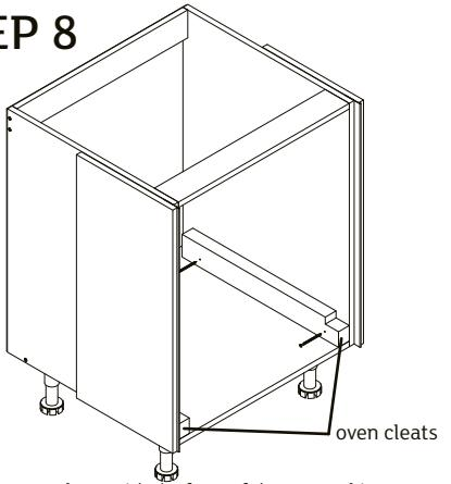
Align the oven cleats with the front of the oven cabinet.
