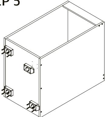
Screw the base plates for the adjustable legs in position.
