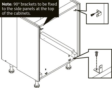
Attach the 90° brackets to the cabinet at the top and bottom using the screws provided.
