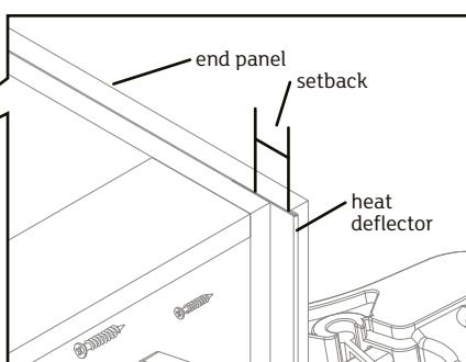
Place the heat deflectors either side of the cabinet so they protrude 20mm. Attach end panels to either side of the cabinet to hold the heat deflectors in place.
