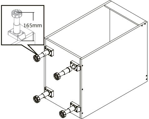
Set the height of the adjustable legs to 165mm.
