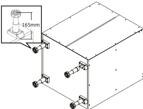
Attach legs to base plates. Set the height of the adjustable legs to 165mm. Repeat for the remaining 3 legs.
