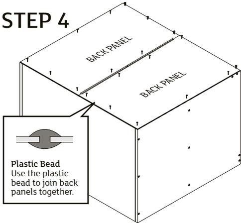
Nail back panel onto the side panels, base panels and fixed shelf. Screw the back panel into the top support rail.
