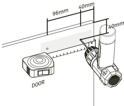
Place masking tape on both sides of the door where holes will be drilled to avoid chipping. Pre-drill using 4.5mm drill bit.
