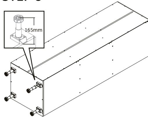
Attach the legs to the base plates. Set the height of the adjustable legs to 165mm.
