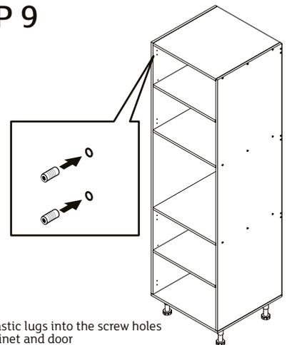
Tap the plastic lugs into the screw holes on the cabinet and door
