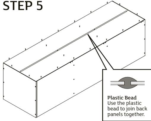
Nail back panels onto the top panel, base panel, fixed shelves and support rails.
