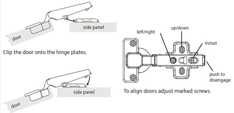
Clip the door onto the hinge plates.
